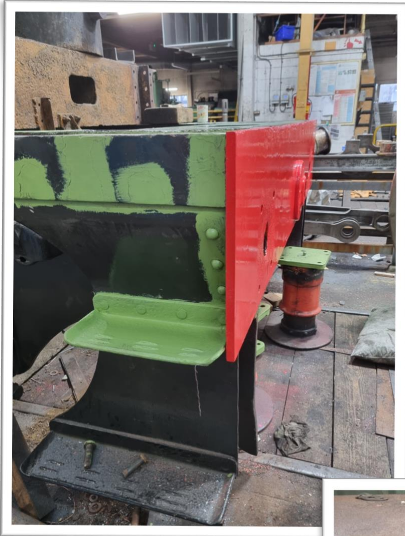
Left: Rear buffer beam and new dragbox of tender chassis, at Sheffield Park. Photo :Steve Pilcher
