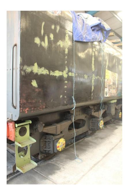
Other recent work, has included loosening the running plate bolts, this is to reduce the amount of work and help have some of the front end prepped for the move into the workshop, more about this will come in future articles. Work has also continued on wire brushing and cleaning the rust within the water tanks, below is an image of the PPE working well, with Andy!
