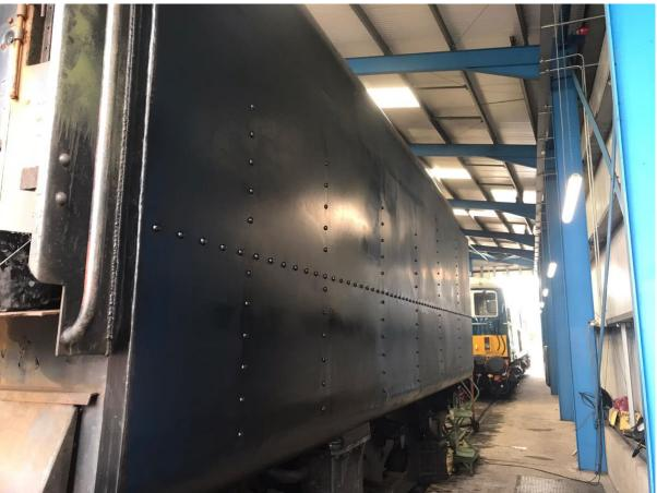
The tender plates have been removed, ready to be cleaned and painted, also removed was the filter lid which has been cleaned and coated in primer. The fall plates have also been removed, although quite a challenge to the team at the working party, which required a lot of heat from a blow torch, impact engineering. The team found that a number of bolts had seized up and later on a hand grinder was used to smooth out the edges of they were lethal.
