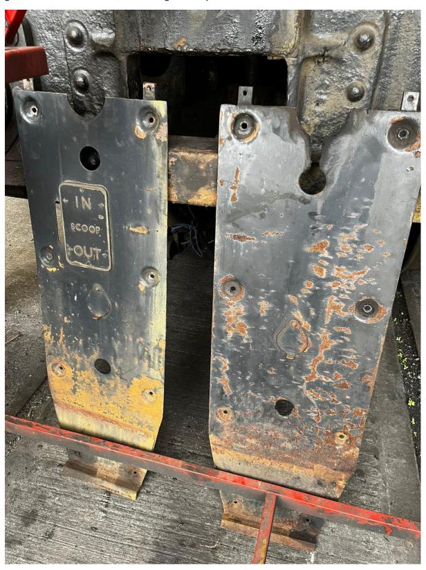
The buffer beam has received a large amount of work, the boot plates have been removed, sand blasted before having primer added onto it. It is the hope of the team, whilst continuing to raise funds whilst using 'Sustainable Funding' to have the tender completed by the end of the year.
