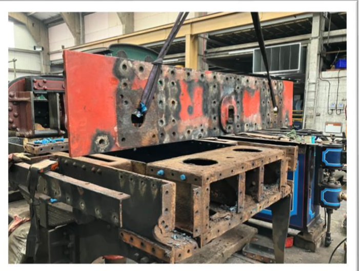
Left: View of the top of the main section of 541's rear dragbox, prior to riveting. Photo: Leaky Finders
