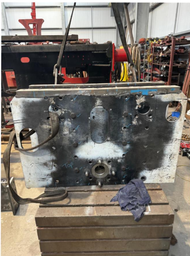
Left: View of the top of the main section of 541's rear dragbox, prior to riveting. Photo: Leaky Finders
