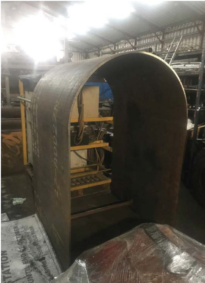
The new firebox outer wrapper plate for Fenchurch. TOM JAMES
