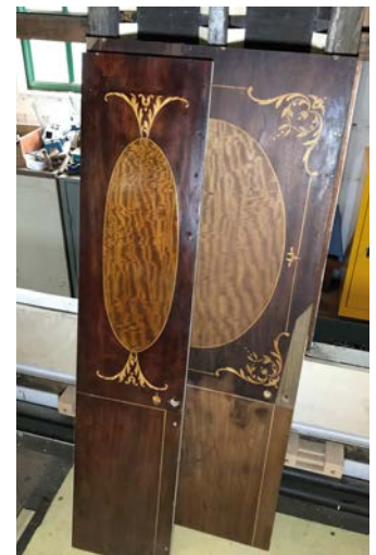
A sample of the skilled work on Pullman Car 54 taking place to stain (so that they all match) and then French polish the new and repaired marquetry panels.
