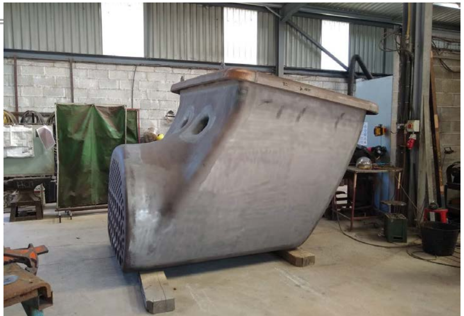
The complete inner firebox for Blackmoor Vale at South Devon Railway Engineering. JOHN FRY
