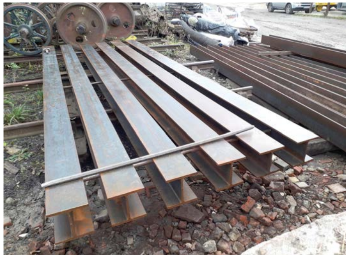
Old and new: Two old wrought iron beams versus 15 new to support each train. BOTH: JON GOFF
