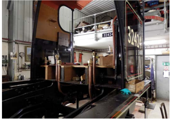
Although the background is rather cluttered the steam feed, delivery and (unseen here) overflow pipes have been made up and fitted to the injectors.
