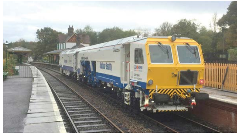
The new tamper on driver training duties at Kingscote station. 'GRIZZ'
