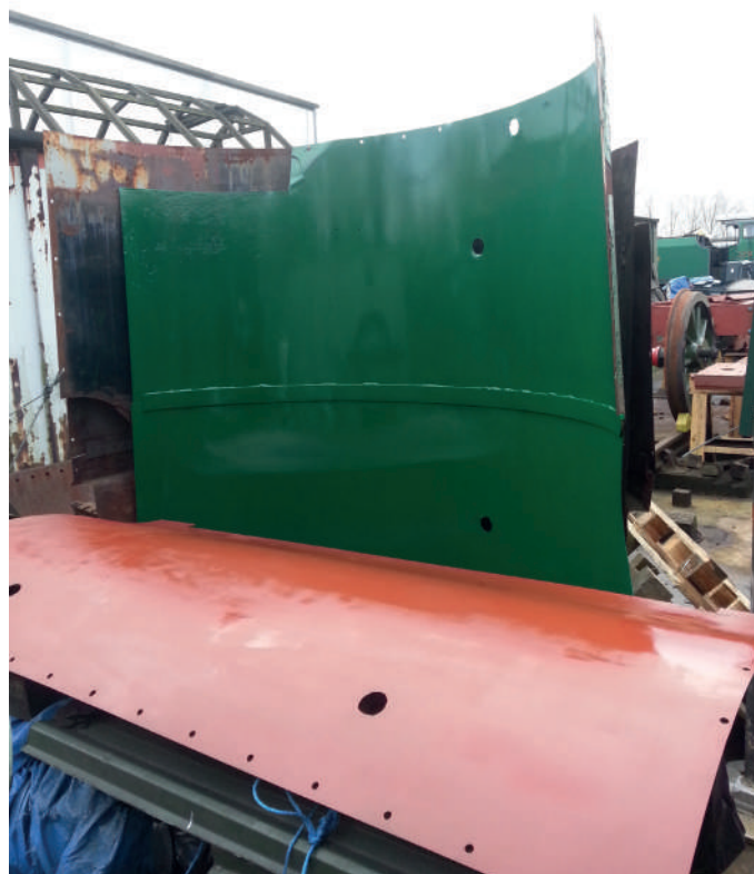
Painting work on the boiler claddings in March 2020. STEVE PILCHER
