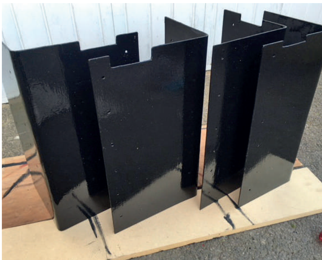
New sheet metal corner plates for Stowe's footplate woodwork. MELVYN FROHNSDORFF
