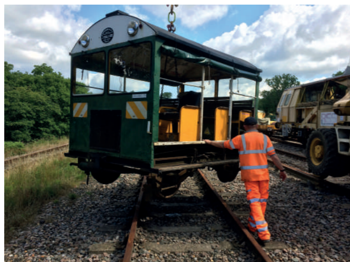
The Wickham Trolley being retrieved and turned at Horsted Keynes Sidings. The conductor rail was isolated! ALI BRUCE
