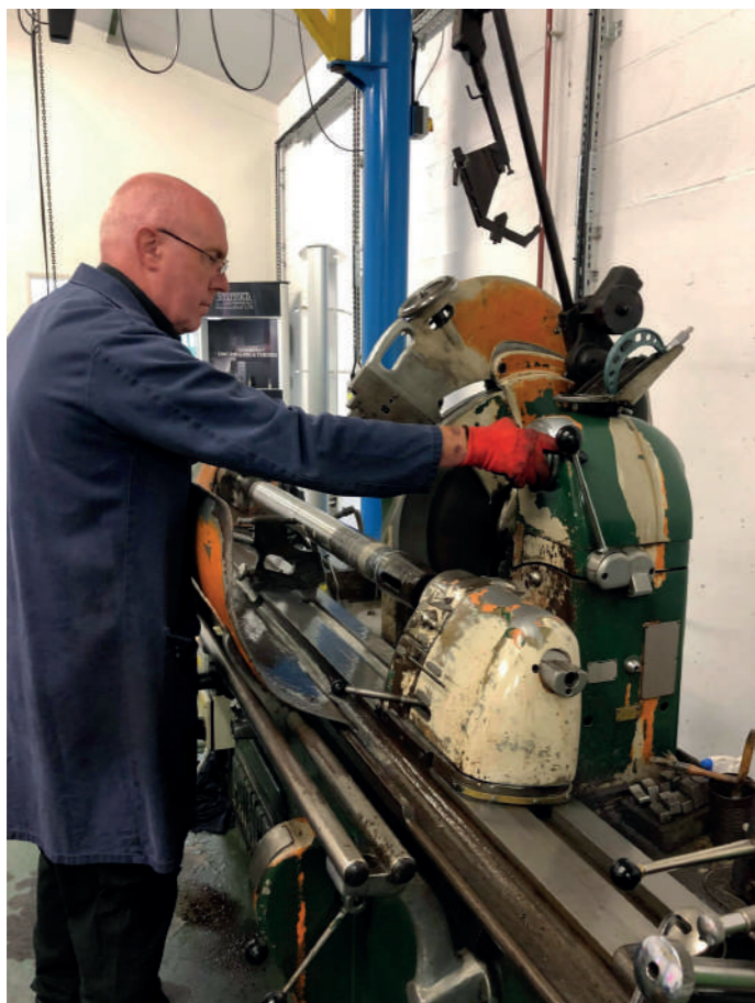
One of Stowe's valve rods being machined. STATFOLD ENGINEERING
