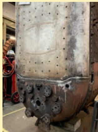
No 72's boiler with new throatplate and backhead fitted, also the new firebox tubeplate offered in for a test fit. HENRY MOWFORTH
