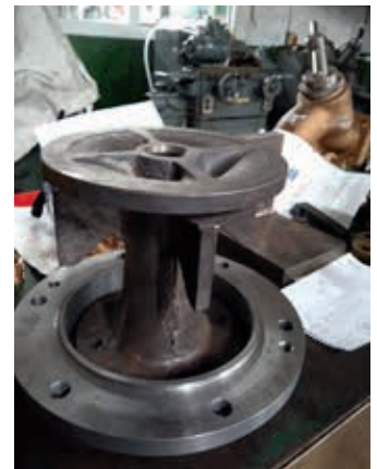
Regulator main valve body. STEVE HECKFORD
