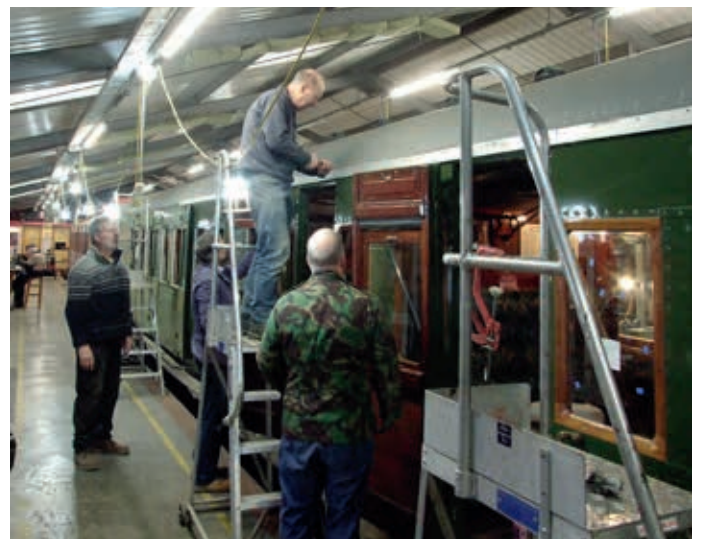
No 3687's gutter is also being fitted on this side.
