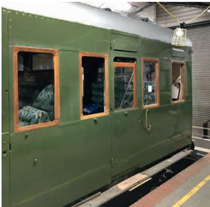
Maunsell Hastings Brake No 3687 is up to fourth (and final) topcoat at the south end of the compartment side, so the first of the quarterlights have been fitted.
