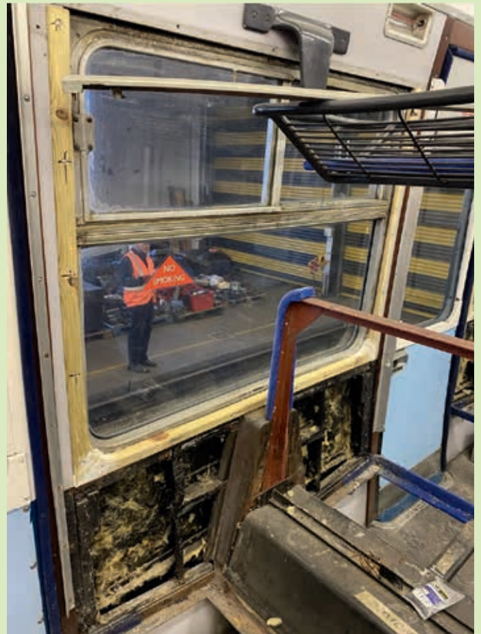
Interior window frame repairs underway.
