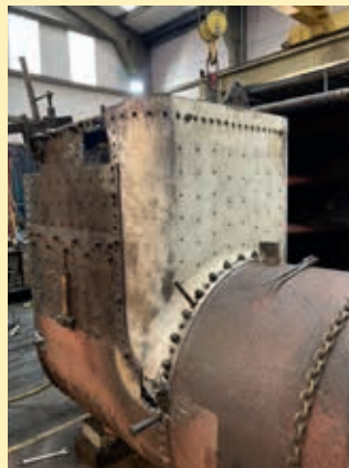
No 72's boiler with new throatplate and backhead fitted, also the new firebox tubeplate offered in for a test fit. HENRY MOWFORTH
