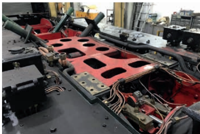
View above the frames, looking towards the back end of the loco, showing the middle engine and valve gear in place, and the numerous lubrication pipes running from the mechanical lubricators mounted on the running plate. TOM JAMES
