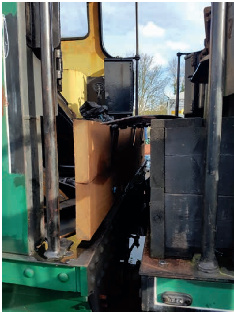
Stowe's new cab fall plate timbers. STEVE PILCHER
