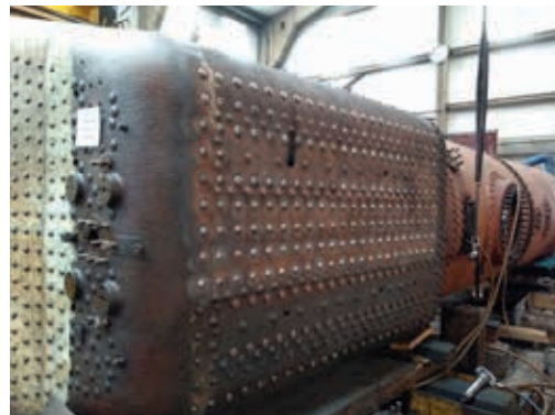
The firebox with the crown stays in situ. JOHN FRY
