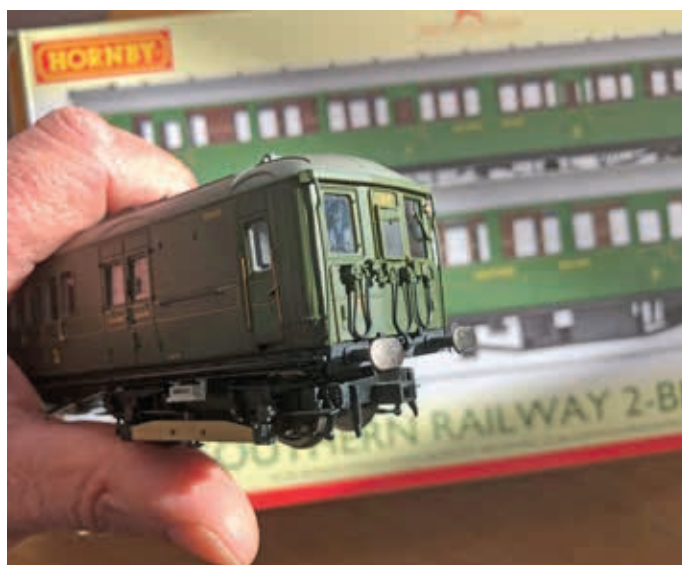
The cab ends are crammed with jumper cable detail.
