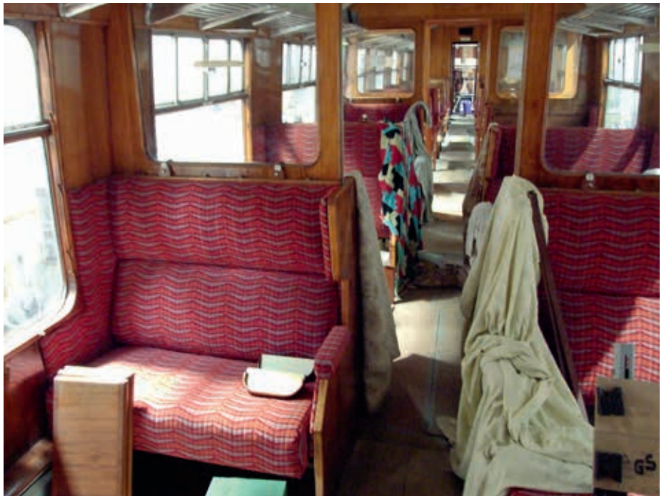
The laying of lino means that the final interior fit of No 4754 can now proceed faster towards completion. The southern saloons, seen here, are largely complete, and the seat frames are also in place in the northern half. This is the first of our carriages to be trimmed in reproduction early-BR 'Boomerang/Aeroplane' moquette, appropriate to this relatively early Mk.1.
