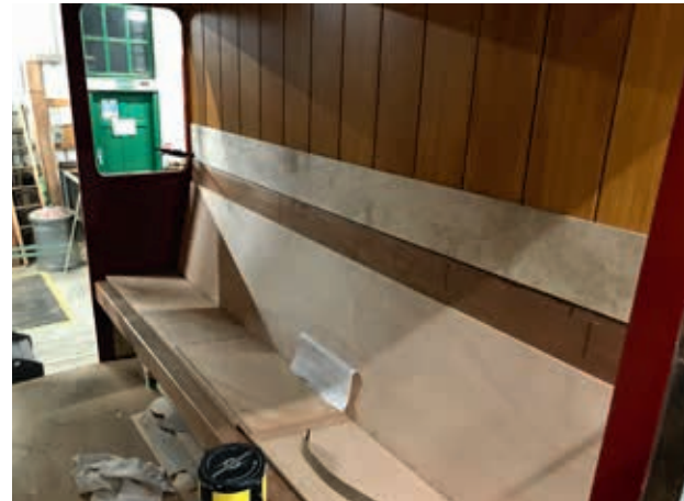
The prototype seat base and back sub-structure for LBSCR Stroudley/Billinton full third 'Betty' (No 328) is being made by John Coleman, and is seen here prior to having upholstery applied by our trimming team.
