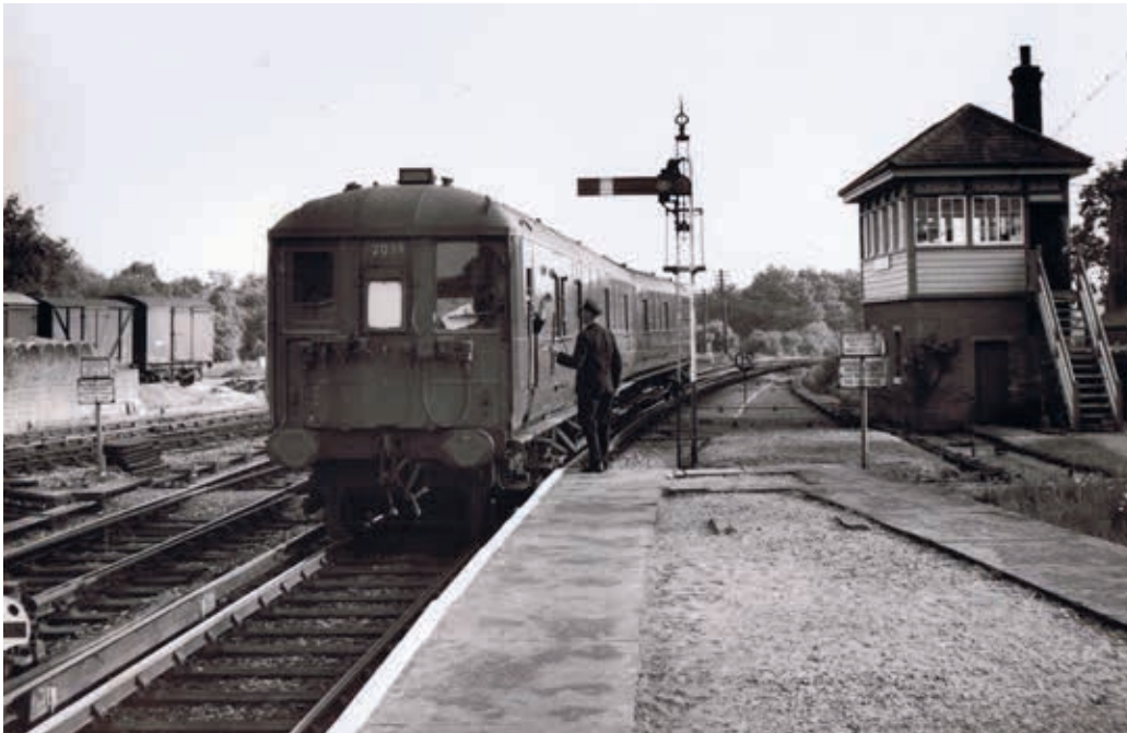
The signalman at Horsted Keynes receives the single line staff from the driver of 2-BIL No 2309 as it approaches the station from Ardingly. The driver will now have time to read his newspaper, propped up against the window, before returning to Seaford. BLUEBELL ARCHIVE
