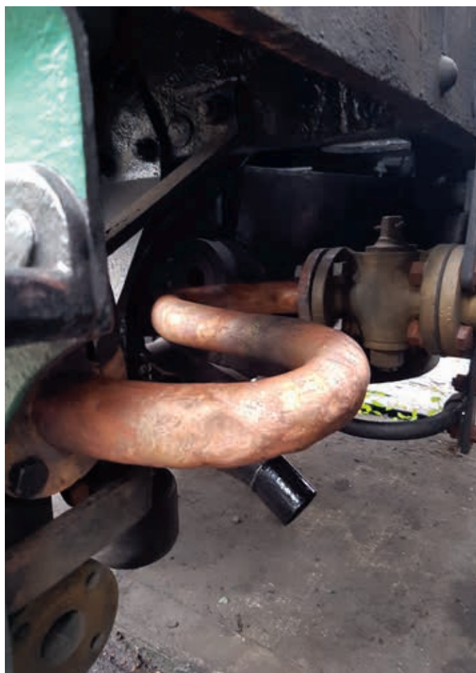
Stowe's refurbished pipework being re-instated underneath the cab. MELVYN FROHNSDORFF
