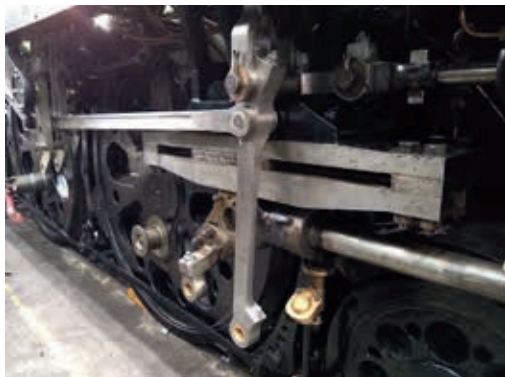
Combination lever and radius rod. JOHN FRY
