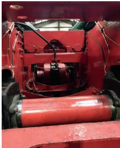
Looking forward between the frames on Sir Archibald Sinclair showing the trailing driving axle; middle crank and big end; and some of the lubrication pipework. TOM JAMES
