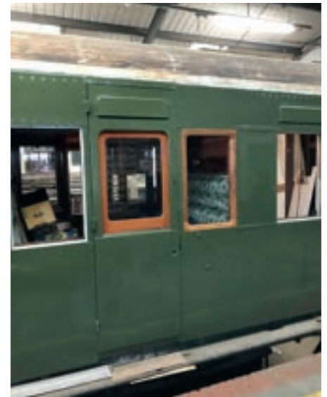
Externally, on No 3687, more paint has been applied to both sides, ventilator bonnets have been fitted and the door trim is ever more complete too. The canvas for the roof is on order.
