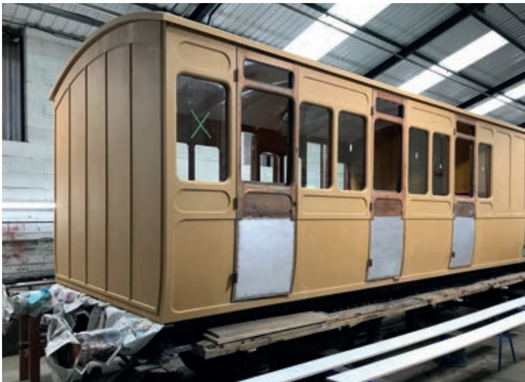
Stroudley Brake, No 949 of 1881, now has seven of its ten doors panelled.
