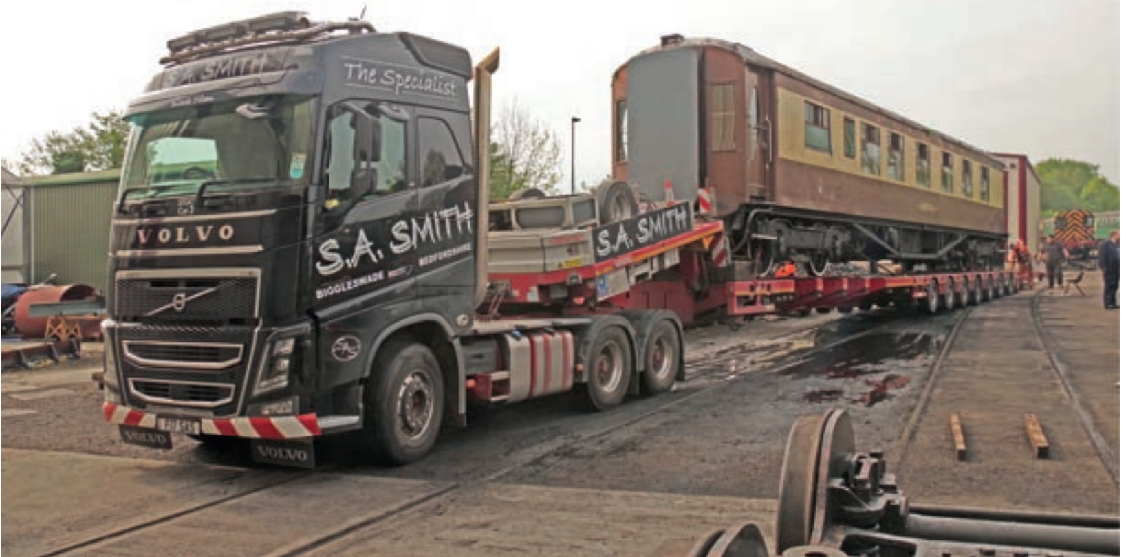
Aquila ready to be unloaded at Sheffield Park on 28 May. Note the advanced trailer being used; prior to unloading the bed of the trailer is raised at the front so that there is only one change of gradient, where the ramp meets the ground. B246
