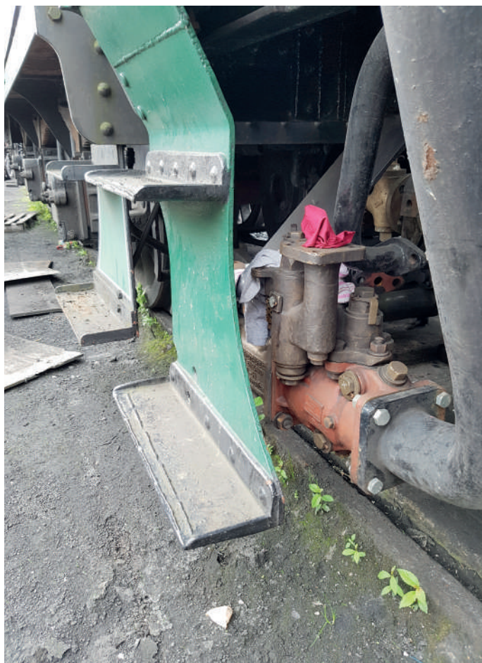
The overhauled exhaust steam injector in place under the cab. STEVE PILCHER
