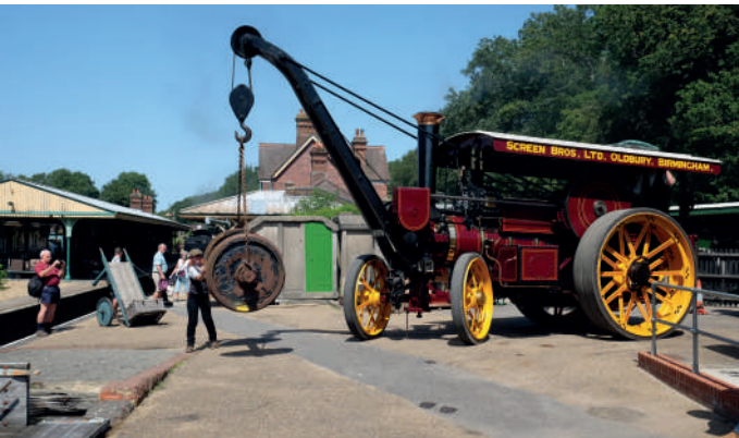
Burrell crane engine No 3197 of 1910 Old Tim on the cattle dock on Horsted Keynes giving a demonstration of lifting wheelsets into a truck.
