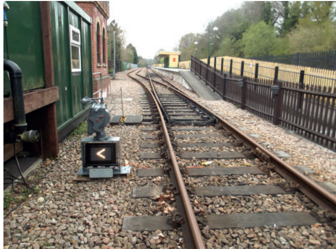
The Pickering indicator at East Grinstead, enabling loco crews to confirm the point position when running round.
