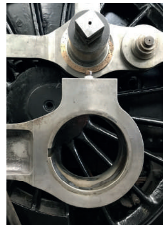
The new bronze casting before machining. TOM JAMES
