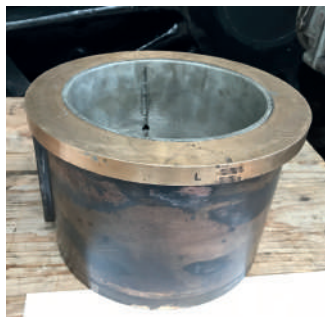
Camelot's big end bearing in worn condition. TOM JAMES
