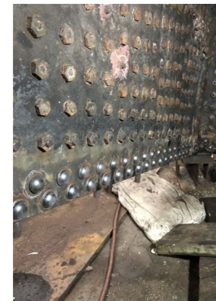
Boiler work on No 73082 Camelot includes the refurbished fountain ring rivet holes and new rivets fitted. HENRY MOWFORTH
