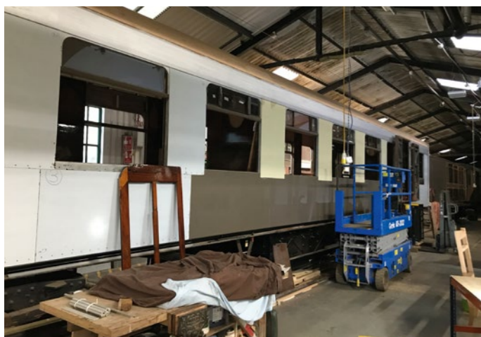
The exterior of Car No 54 is starting to be painted (seen here partly in undercoat) in January. RICHARD SALMON
