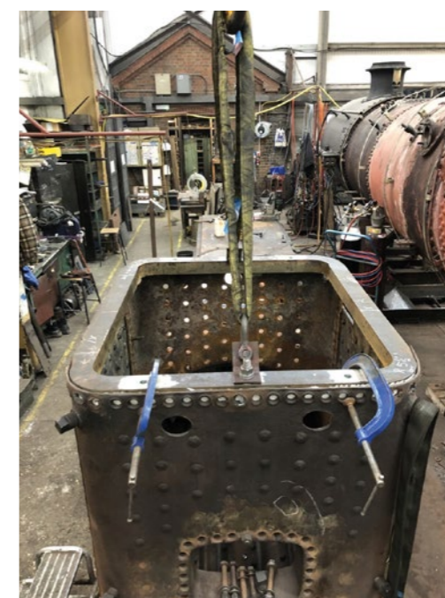
Two views of the trial fitting of the new foundation ring on No 72 Fenchurch . HENRY MOWFORTH
