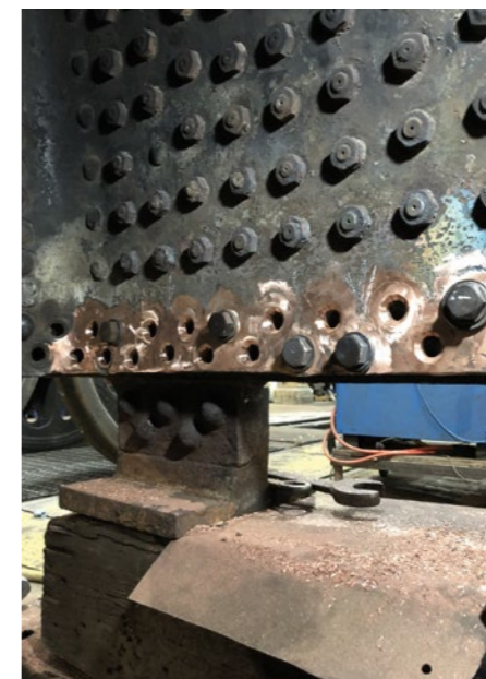
Boiler work on No 73082 Camelot includes the refurbished fountain ring rivet holes and new rivets fitted. HENRY MOWFORTH
