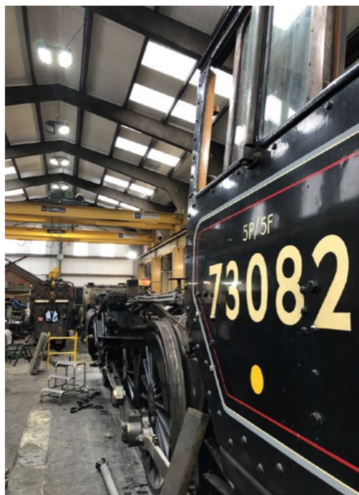
Many of the recent tasks in the locomotive workshop have been centred on a full boiler inspection and overhaul for No 73082 Camelot , with the intention of obtaining a new ten-yearly certificate. HENRY MOWFORTH
