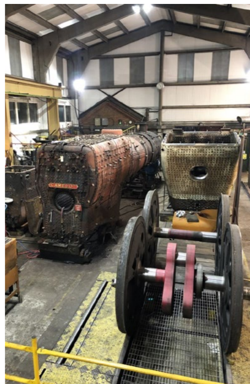
Camelot's boiler (left) having been lifted from its wheels. HENRY MOWFORTH
