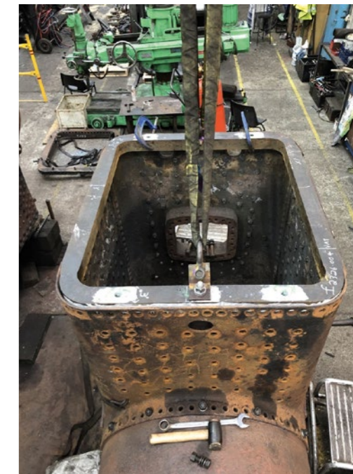
Two views of the trial fitting of the new foundation ring on No 72 Fenchurch . HENRY MOWFORTH
