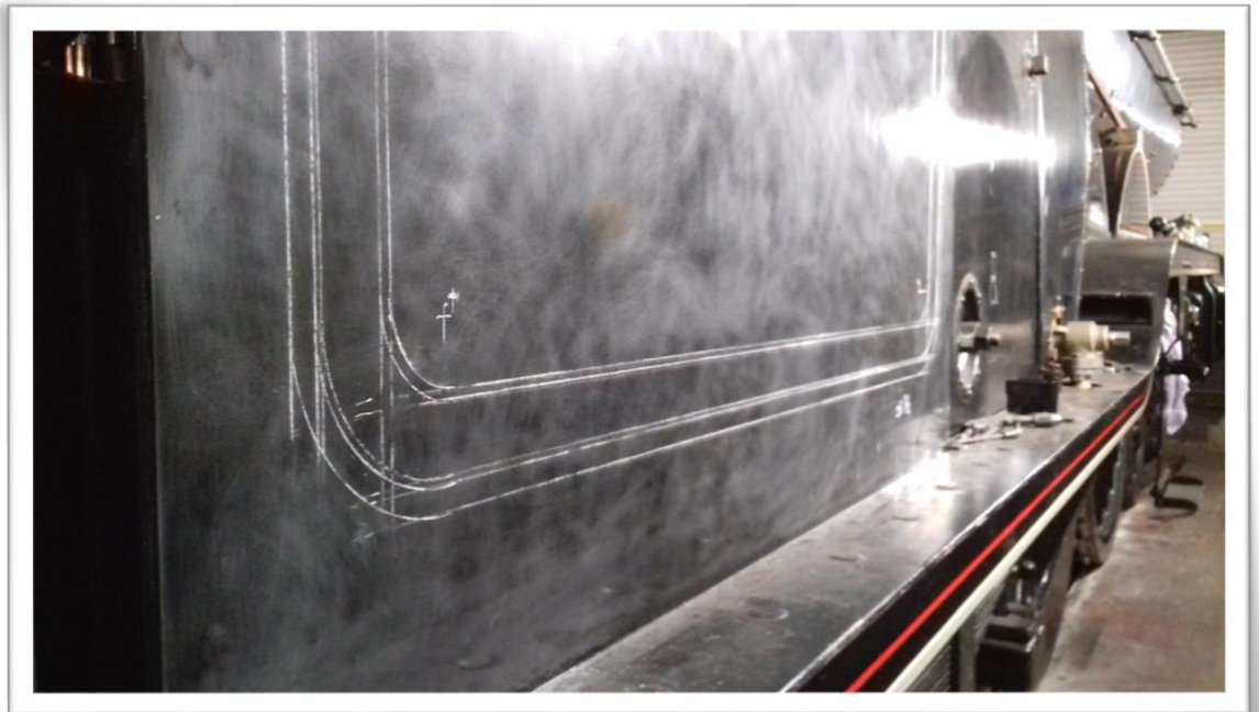
Right: Tony Funnell's chalk guidelines ready for the final lining and lettering on the right hand cabside. The left hand one was done some years ago as that was on view to visitors to Atlantic House. The right hand nameplate sponsored by Guy and Robin Cooper of Swadlincote is also ready for bolting on.
