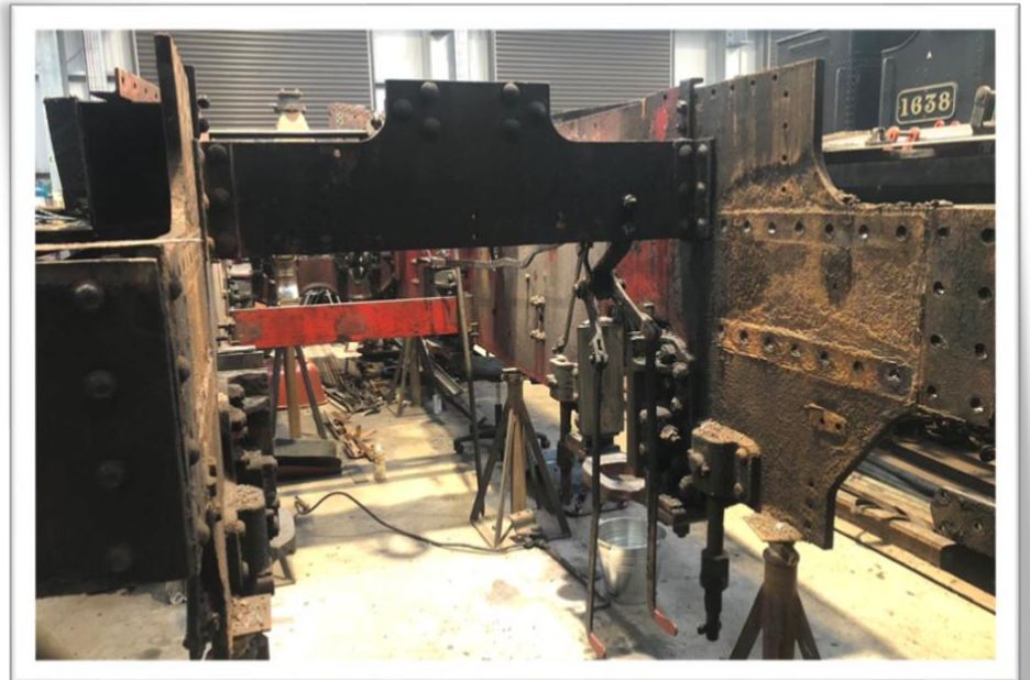
Right: The rear of the loco's frames, showing where the dragbox has been removed.
