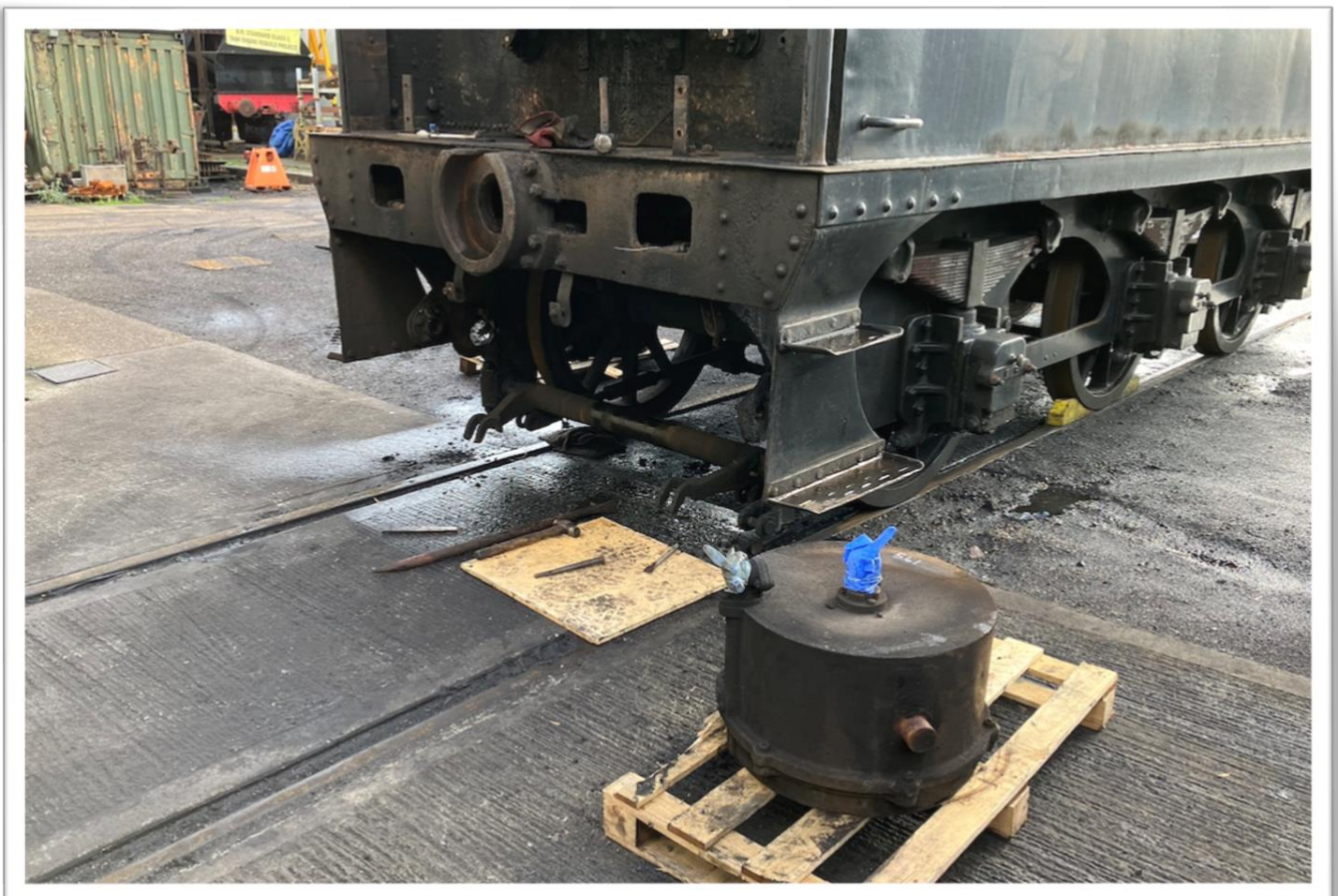
Above: One of the tender's brake cylinders, having been extracted from under the tender.
