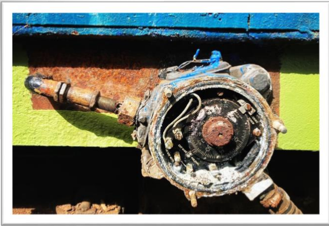
Above: Corroded speedometer
