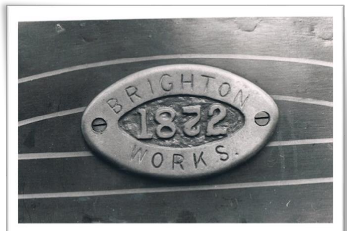
The distinctive works plate, with an upside down '2' acting in place of a '7'.
