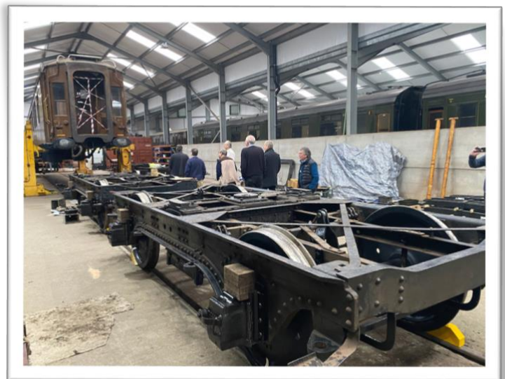
Inside the maintenance section of OP4, with ‘Fingall’ undergoing maintenance to its running gear. The roof here is raised to allow lifting of carriages clear of their bogies
