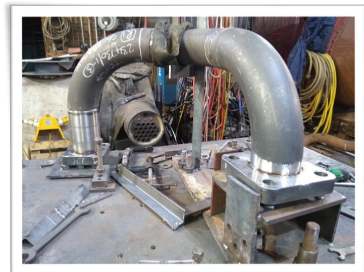
Top to bottom: Progress on Fenchurch's boiler – new front ring and smokebox tubeplate. Boring the cylinders for No. 541. New steam pipes for No. 541
