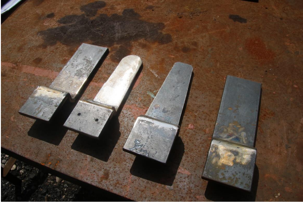
Above four of the six lamp brackets required for the back of the bunker under construction and they will soon be fitted.
