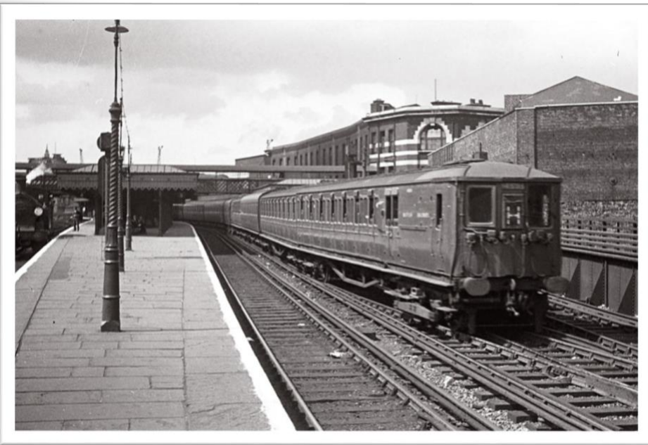
4-SUB 4535, standing at London Bridge forming the 2.38pm Charing Cross - Hayes via Lewisham Service on 17 July 1949. The leading motor brake is an arc-roofed LBSCR bodied vehicle whilst the third vehicle is a Bulleid ten compartment 'six-a-side' augmentation trailer. These trailers were added to many three-car units in the closing days of the Southern Railway and the dawn of British Railways to form 4-SUB units although these all-steel modern trailers stuck out like a sore thumb against the pre-grouping bodywork of the remainder of the units. Photographer John J Smith.
