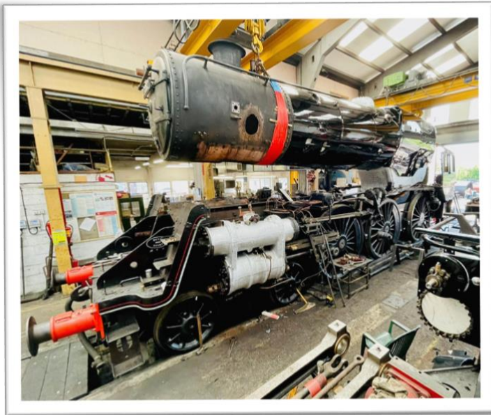
(Above): At Sheffield Park, the reassembly of 'Camelot' is continuing, with the boiler being lifted back into the frames on 31 May. Photo: Henry Mowforth.
