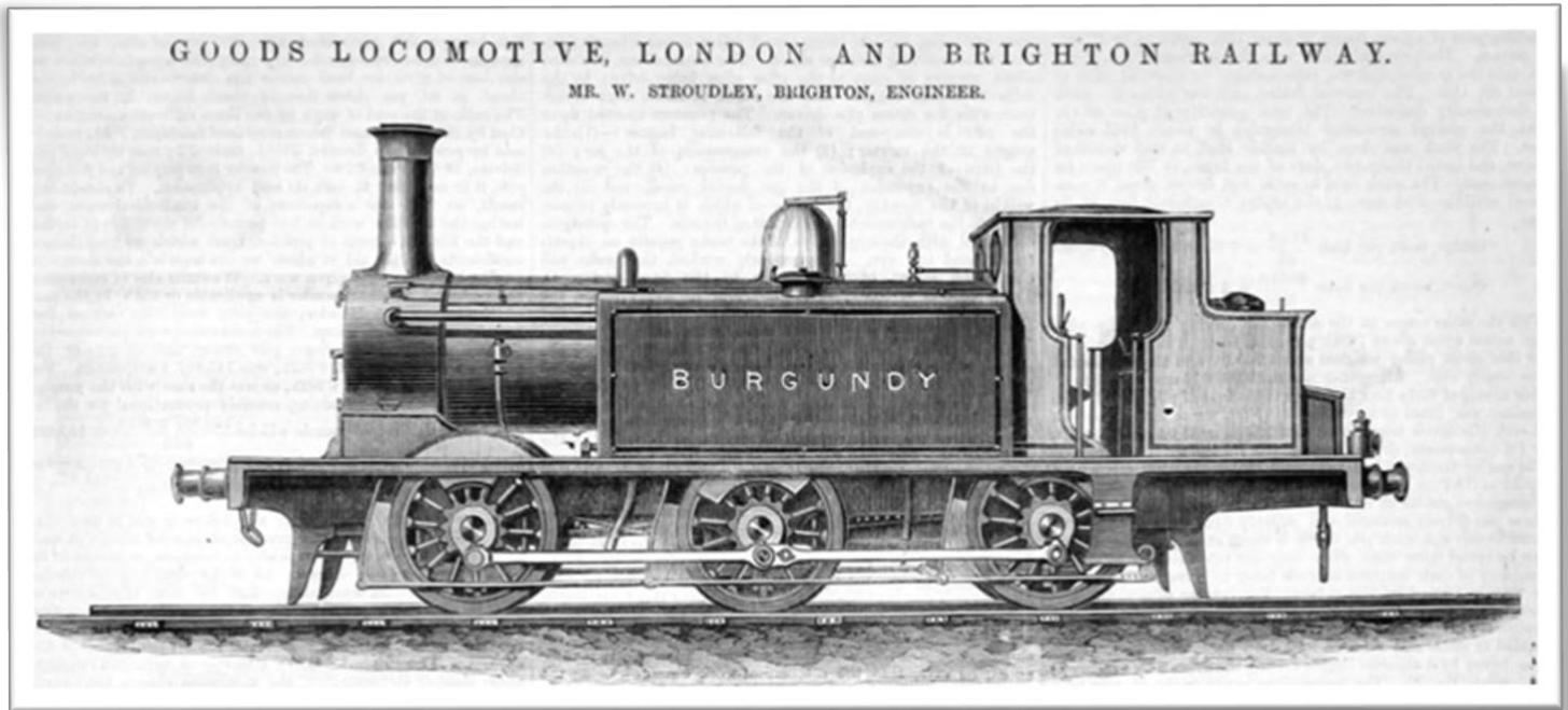
LBSCR E class goods locomotive "Burgundy", as originally built. Note the wooden brake blocks, and absence of any brake apart from a handbrake. Like 'Fenchurch', this particular locomotive had a rather peripatetic life and is now also preserved, at the Isle of Wight Steam Railway. Illustration: Grace's Guide to British Industrial History
