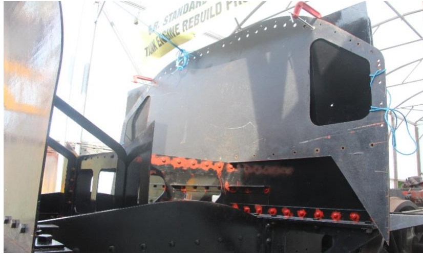
Top Section of Cab End Panel Awaiting Assembly
