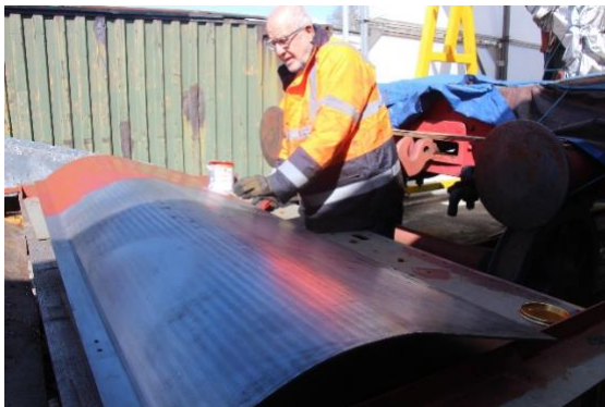
Protective Painting off the Rear Bunker Panel
